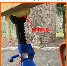
to make the reading less critical and jerky. We now use a polyurethane round bar that has been hollowed, to act as a spring. It is placed between the bar and the fixed jack.
