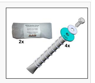
**Installation** The installation requires drilling a 7/8" hole 6" deep into the asphalt and the gravel below it. The grout is supplied as a cement powder. It requires the addition of water to activate it. The hole is filled with the grout and the anchor is dropped in. The anchor is ready for use in 15 minutes .
