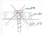
method will not use the bolt to capture the sill, as the head of the anchor is *above* the plate. It also will prevent the removal the of the sill plate and the plate will be permanently captured by the anby the *bolt* that at-
